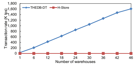
Figure 18: Performance comparison between THEDB-DT and H-Store. The number of cores is set to 46.
